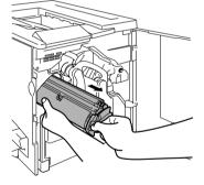
Each toner cartridge has a colored end that corresponds to a color inside the cartridge slots. Always install the toner cartridge in the slot of the same color.
